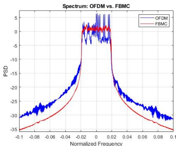
**Fig. 8.** Comparison between the OFDM and FBMC Spectrum.
